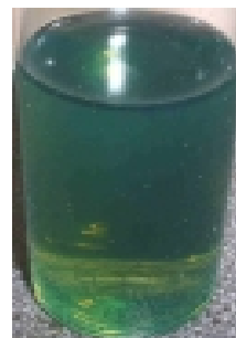
OMP 7000 after air agitation: - obvious flocculation - Concentration: 41%
